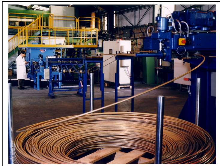
Fig 7 : Horizontal Continuous Casting – Copper Alloy Wire Rod 12-120mm Diameter
