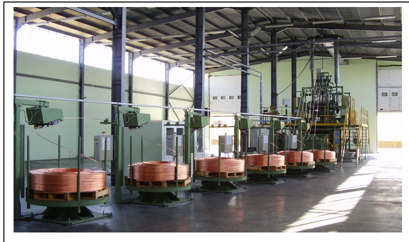
Fig 4 : Rautomead RS 3000 integrated melting and Casting machine. 6 strands, 5,500 – 6,000 tonnes/year
