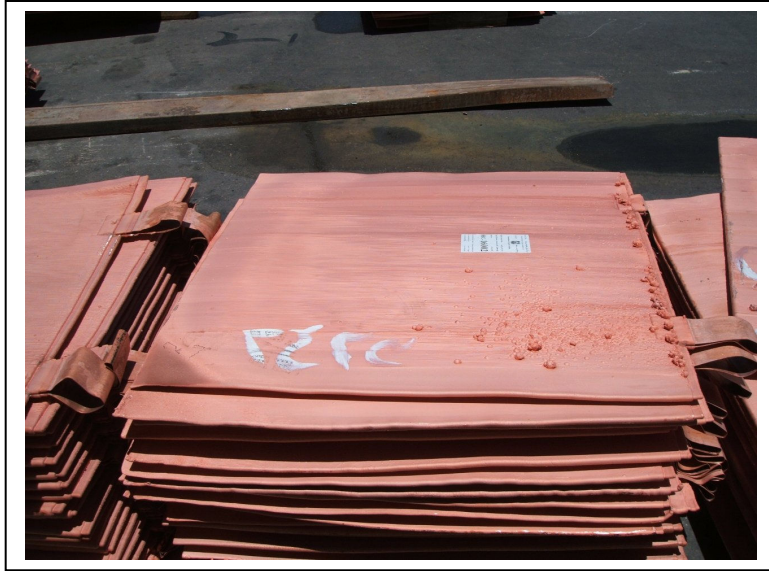
Fig 2a Grade A - electrolytically refined full deposit cathode.
