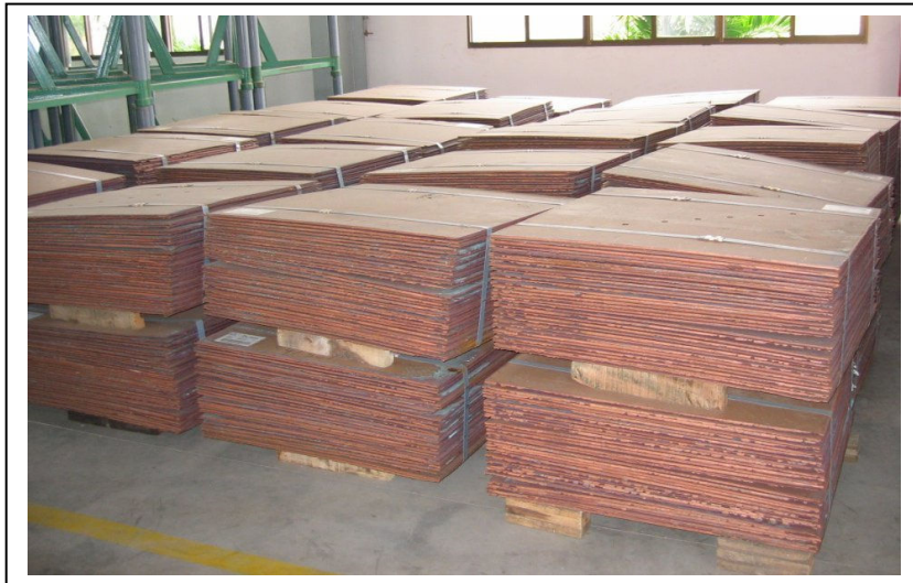
Fig 2b Grade A - electrolytically refined ISA Process™ cathode
