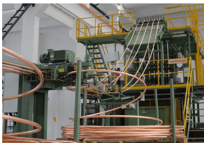
fig. 3 Rautomead RS 3000/5-CuMg Casting Machine
