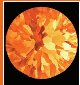
Longitudinal Section 30mm CuMg As-cast Rod
