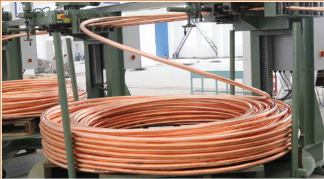
Coil Formation – 3 Tonnes Capacity
