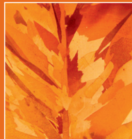
Transverse Section 30mm CuMg As-cast Rod
