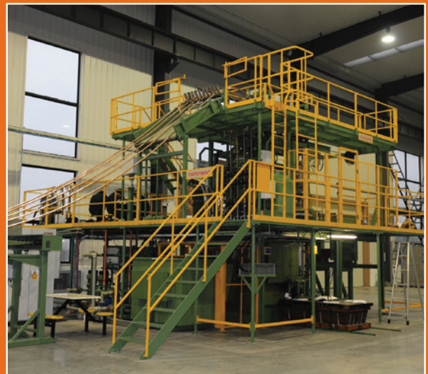
RS 3000/5/CuMg Continuous Casting Machine
