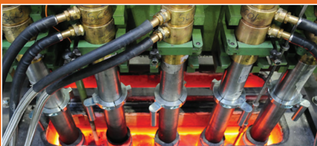
Casting Dies and Supercooler Assemblies
